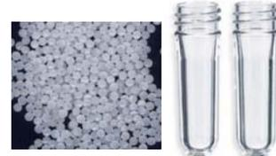
At a plastics factory the oil is transformed into plastic pellets then bottle pre-forms.
