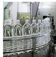
The bottles are brought to the bottling plant where they are filled with water.
